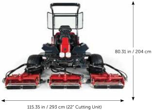
115.35 in / 293 cm (22" Cutting Unit) 124.41 in / 316 cm (26" Cutting Unit)
