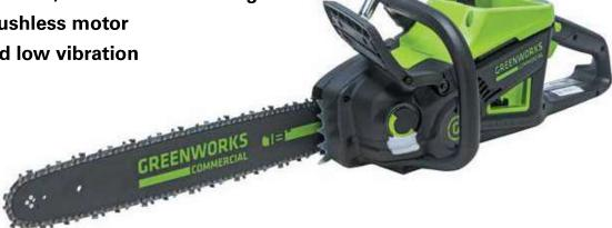
Cut faster than petrol every time with the GREENWORKS® 82V 18" commercial chainsaw. The brushless direct drive motor and cutting system combines 3.4Nm of torque and constant power to provide optimal cutting performance while decreasing noise and vibration and gives you all the power of a 55cc petrol engine with a faster cutting speed - 2.7kW/3.6hp output.
