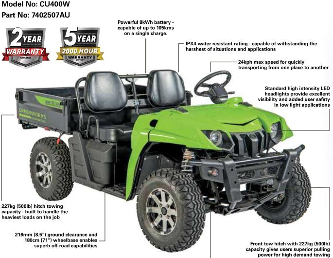
Independent, dual A-Arm type premium suspension for a comfortable ride on rougher terrain
