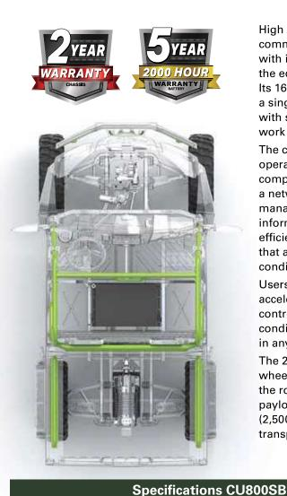
High powered performance you can count on. The GREENWORKS<sup>®</sup> commercial utility vehicle (UTV) is designed to go the distance with its powerful 16kW max gTRON<sup>™</sup> drive system, operating with the equivalent power of a 31hp / 496cc displacement petrol engine. Its 16kWh battery module provides up to an impressive 120km on a single charge for all day use. This vehicle is up for any challenge with superior off-road performance and on-demand 4WD for a true work utility experience.
