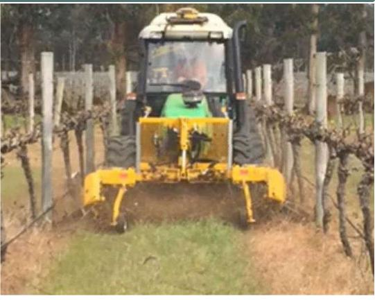
Width setting from 2.2m to 4m is achieved by two synchronised hydraulic rams.
