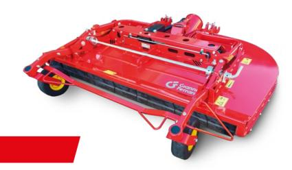
**Blade transmission** by mechanical reducers with spheroidal cast iron boxes and helical bevel gears in an oil bath **is robust and reliable**. The discs with **shockproof swing back blades** protect the transmission against impact with foreign objects left in the grass.
