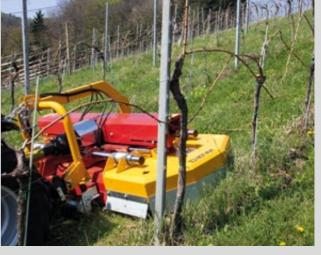
Thanks to the pendulum frame, the weight of the entire rotary mower is optimally transferred to the tractor.
